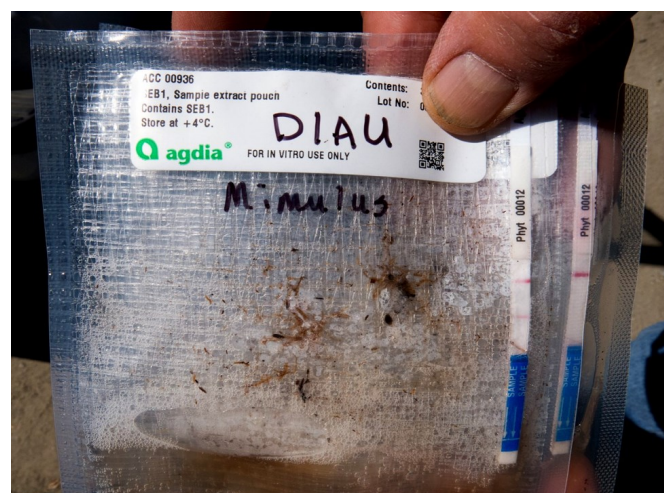
Fig. 10. Immunostrip test for Phytophthora . Symptomatic roots are sampled, macerated in a buffer test solution and pouch. The test strips inserted in the pouch indicate results in as little as few minutes. Test strips have a magenta-pink-colored “control line” indicating a valid test, as seen in both test strips here. If Phytophthora is detected, then two lines appear: a control line and a “ Phytophthora -discovered” line. You can see the latter line next to the red arrow on the strip to the left (although more weakly) but not on the strip to the right. Photo: S. Tjosvold.
