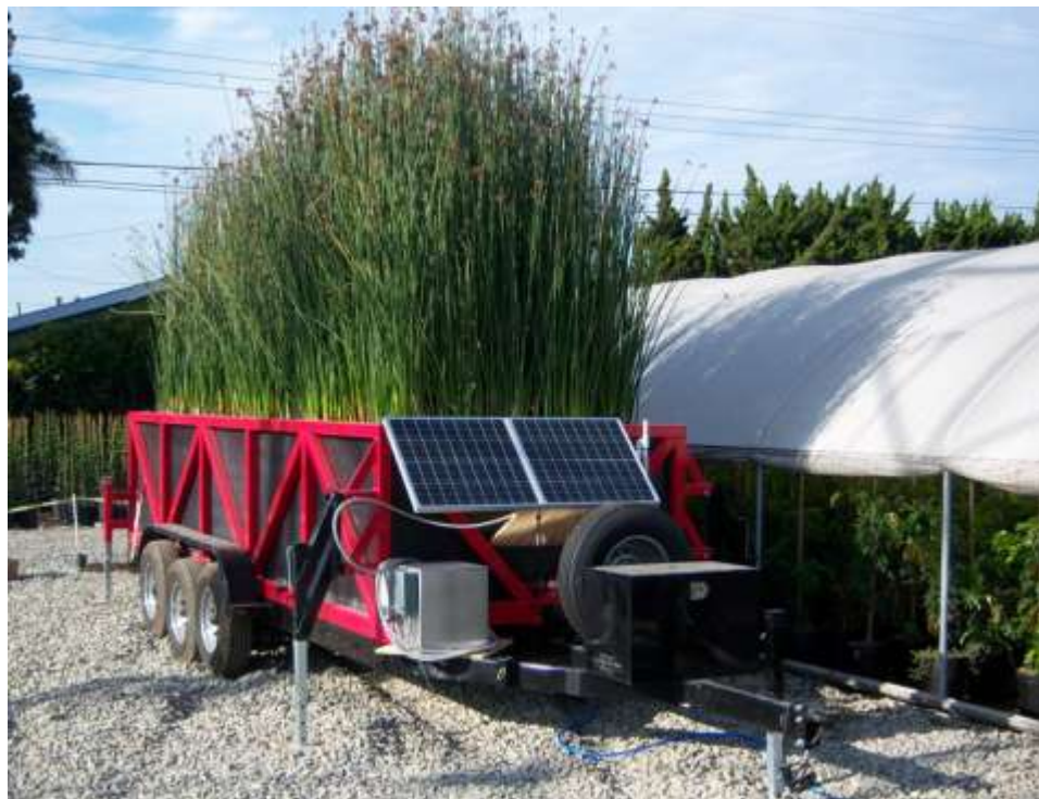
Fig. 3. Portable subsurface flow wetland established with bulrush, water moves through the wetland via a solar-powered pump. Image Jim Welsh.
